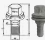
FLAT BOLT WITH WASHER BULLONE PIATTO CON RONDELLA (stainless steel cap)
